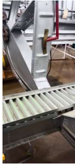
B-24 Liberator bomb bay repair patch (Photo courtesy of Paul Rourke)
