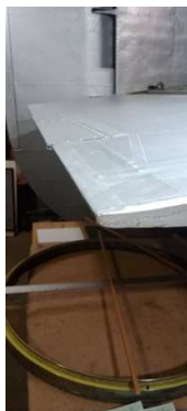
B-24 Liberator Elevator trim tabs manufactured and fitted to tail plane (Photo courtesy of Paul Rourke)
