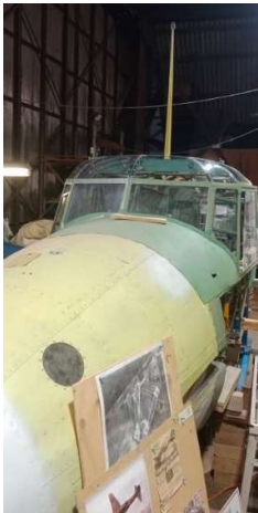
Anson windscreen Plexiglass being installed (Photo courtesy of Paul Rourke)
