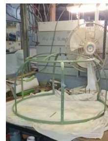
Anson turret dome structure (Photo courtesy of Paul Rourke)
