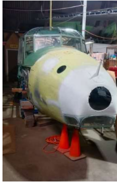
Anson windscreen Plexiglass being installed (Photo courtesy of Paul Rourke)
