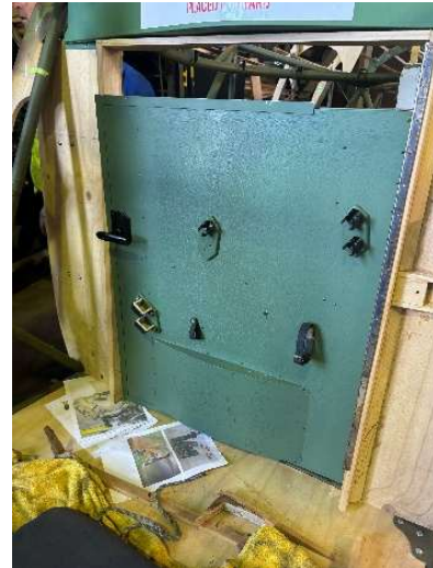
Anson door providing access to the turret, ready for installation
