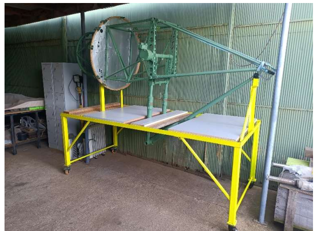
The Avro Anson nose cone and stand for work on undercarriage oleo legs
