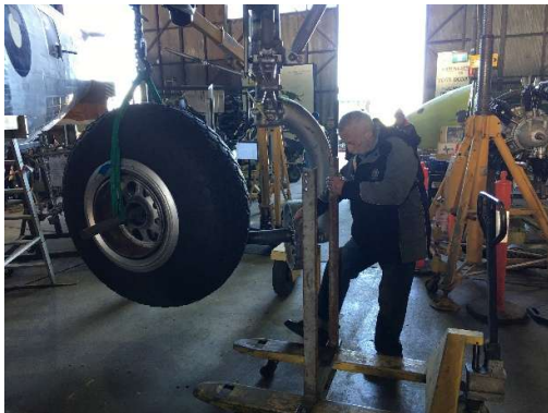
A volunteer helping to prepare the main wheel port side for fitting to the B-24 Liberator (Photo courtesy of John McCrystal)
